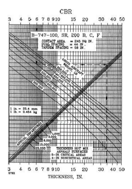
Figure A1.6. Flexible pavement design curves, b-747-100, SR, 200 B, C, F (Source: FAA)
