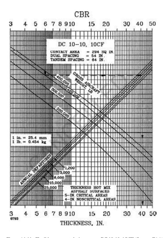
Figure A1.11. Flexible pavement design curves, DC 10-10, 1OCF (Source: FAA)
