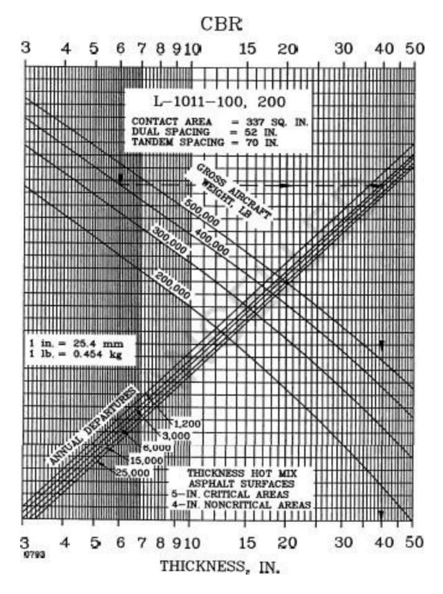
Figure A1.14. Flexible pavement design curves, L-1011-1,200 (Source: FAA)
