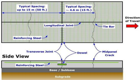
Figure 4.1 Jointed reinforced concrete pavement (JRCP)
