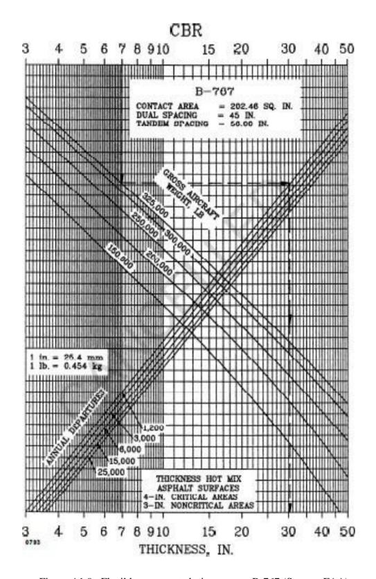
Figure A1.9. Flexible pavement design curves, B-767 (Source: FAA)
