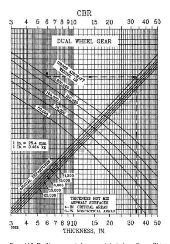
Figure A1.2. Flexible pavement design curves, dual wheel gear (Source: FAA)
