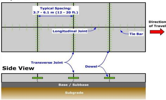
Figure 4.3. Jointed plain concrete pavement (JPCP)
