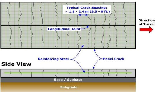
Figure 4.2. Continuously reinforced concrete pavement (CRCP)
