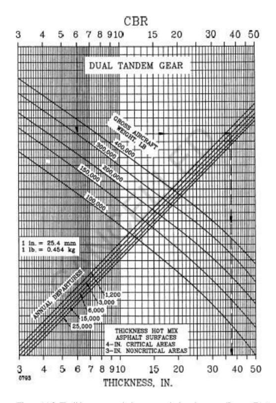
Figure A1.3. Flexible pavement design curves, dual tandem gear (Source: FAA)
