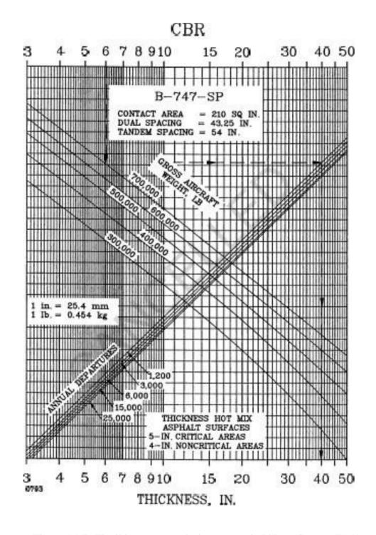
Figure A1.7. Flexible pavement design curves, b-747-sp (Source: FAA)
