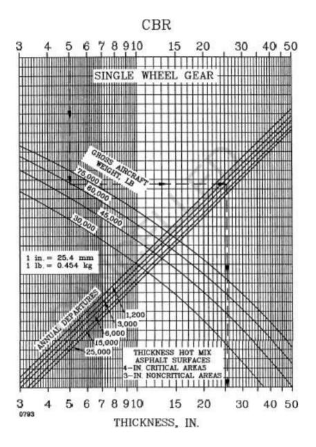
Figure A1.1. Flexible pavement design curves, single wheel gear (Source: FAA)
